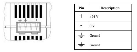
The  $\frac{\perp}{=}$  pins are to be connected using as short a cable as is possible. If the Panel is mounted in a cabinet, the connecting cable should be as short as possible.
